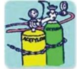
Keep the protective cap in place at all times when the cylinder is not in actual use. Cylinder must be properly labeled with contents and hazard warnings.
